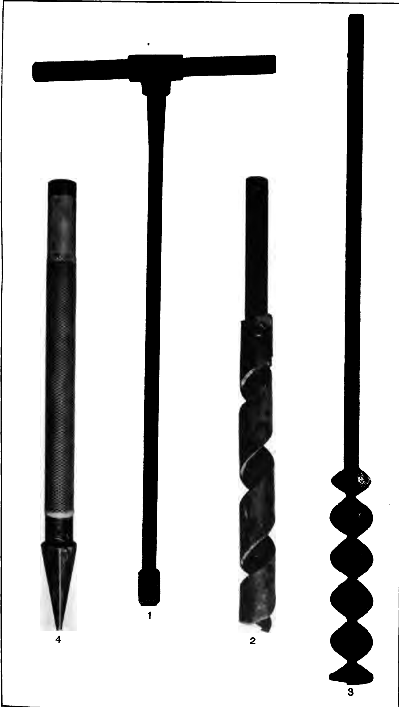
1. SMALL EARTH AUGER; 2, 3. EARTH-AUGER BITS; 4. DRIVE POINT AND SCREEN.
